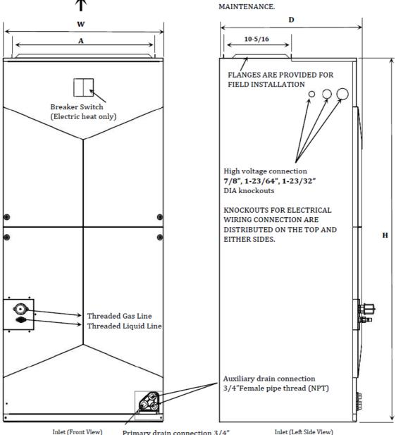
Primary drain connection 3/4" Female pipe thread (NPT)
