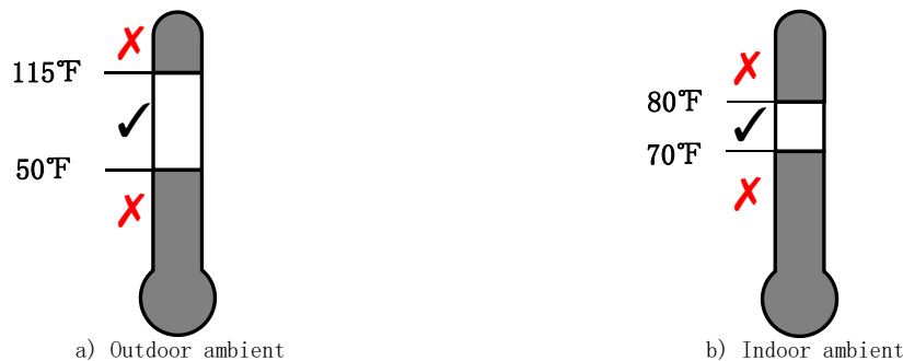
Fig 13-2 Temperature limit for AUTO charge mode
