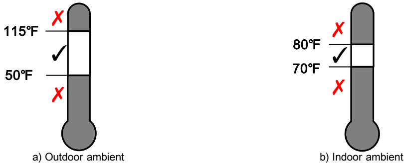
Fig 13-2 Temperature limit for AUTO charge mode
